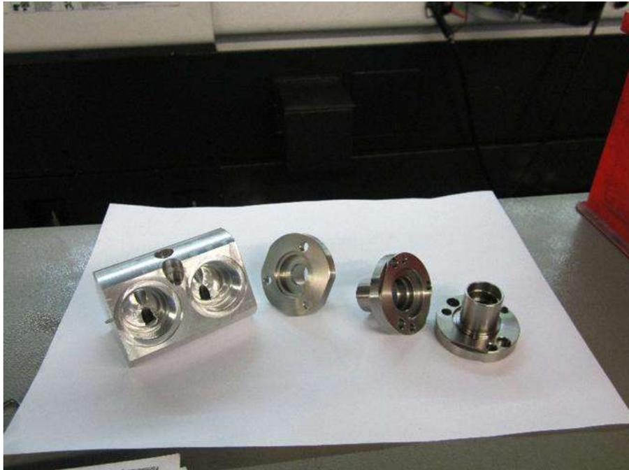
Sample parts, typical of those programmed with GibbsCAM and machined on the Integrex at Pomtava
